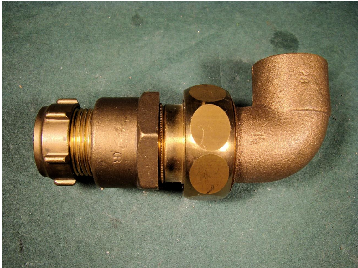
Figure 9 Combination of yellow brass fittings and reddish gunmetal bronze pipe-bend Note the colour difference.
