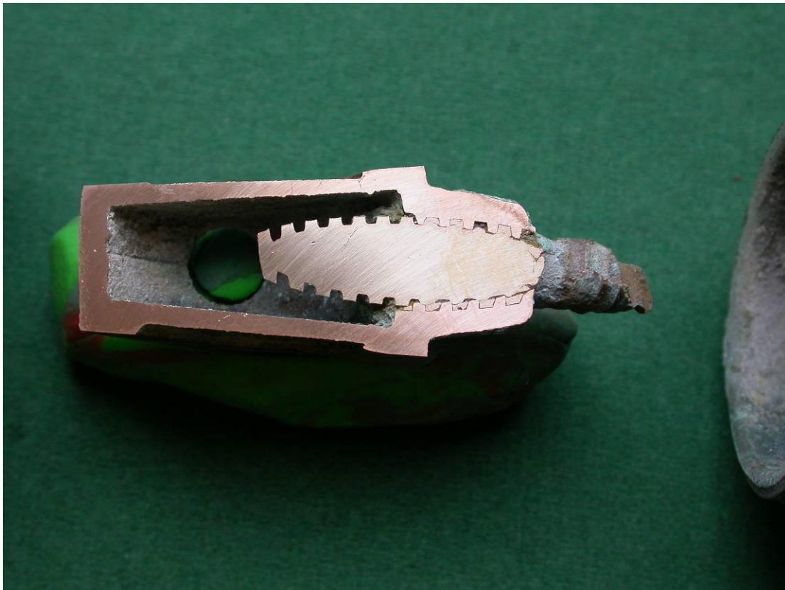
Figure 4 The broken spindle in the stem. The colour difference between the light yellow brass and the red-yellow bronze is obvious here. The brass metal is attacked by dezincification corrosion causing the spindle to jam and break.
