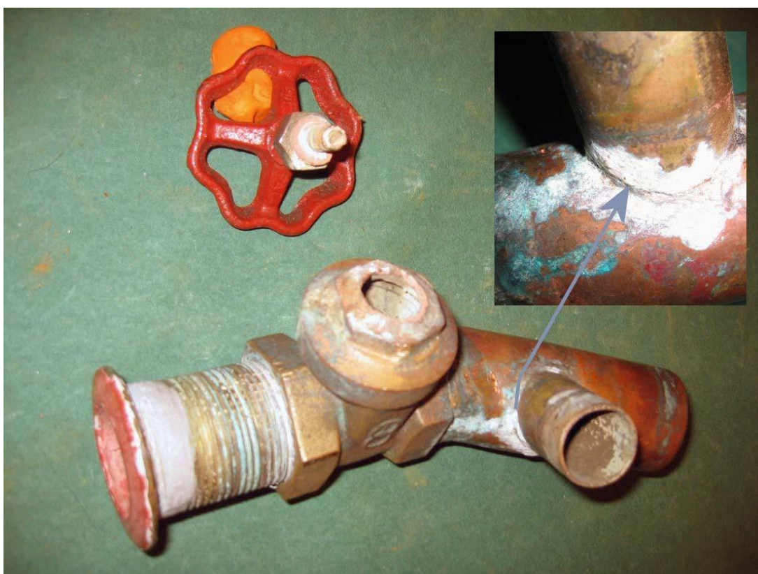
Figure 2 Dezincification and broken gate sea cock valve. The cover has broken off causing a major leak and major ingress of seawater into the boat.
