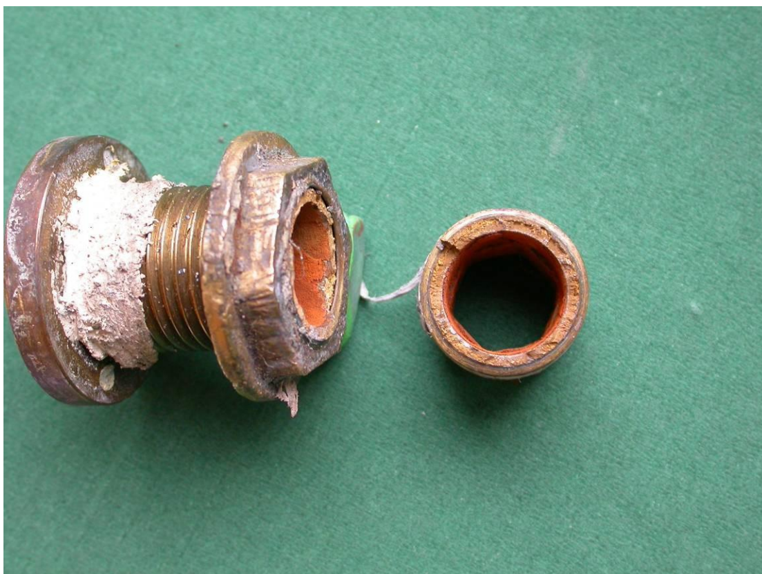
Figure 1 Hull fitting for cooling water, made of brass, broken in the thread inside the boat. Possibly due to ammonia stress corrosion.
